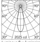
Luminous flux luminaire 647 lm (EXTREME CUT OFF)
