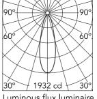
Luminous flux luminaire 625 lm (EXTREME CUT OFF)
