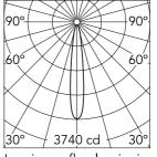
Luminous flux luminaire 412 lm (EXTREME CUT OFF)
