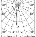
Luminous flux luminaire 448 lm (EXTREME CUT OFF)
