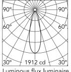
Luminous flux luminaire 592 lm (EXTREME CUT OFF)
