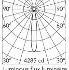
Luminous flux luminaire (EXTREME CUT OFF) 420 lm
