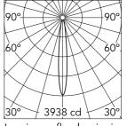
Luminous flux luminaire 344 lm (EXTREME CUT OFF)
