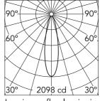
Luminous flux luminaire 544 lm (EXTREME CUT OFF)
