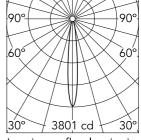
Luminous flux luminaire 332 lm (EXTREME CUT OFF)
