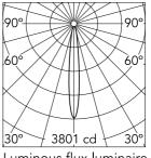
Luminous flux luminaire (EXTREME CUT OFF) 332 lm
