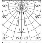
Luminous flux luminaire 474 lm (EXTREME CUT OFF)
