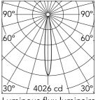
Luminous flux luminaire 328 lm (EXTREME CUT OFF)
