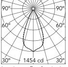
Luminous flux luminaire 780 lm (EXTREME CUT OFF)
