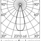
Luminous flux luminaire 741 lm (EXTREME CUT OFF)
