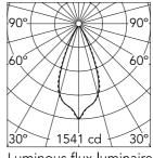
**Emergency** Insulation class h(m) E(lx) D(m) 1541 0.80 385 1.60 3 171 2.40 96 3.19 62 3.99
