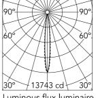
Luminous flux luminaire 751 lm (EXTREME CUT OFF)
