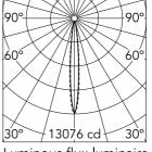
Luminous flux luminaire 724 lm (EXTREME CUT OFF)
