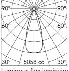
Luminous flux luminaire 2032 lm
