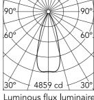
Luminous flux luminaire 1952 lm
