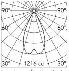
Luminous flux luminaire 705 lm
