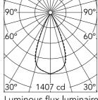
Luminous flux luminaire 764 lm (EXTREME CUT OFF)
