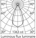
Beam Angle: 45° h(m) = E(Ix)D(m) 1363 0.83 2 1.67 341 3 151 2.50 3.34 85 55 4.17
