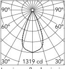
Luminous flux luminaire 716 lm (EXTREME CUT OFF)
