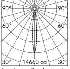
Luminous flux luminaire 801 lm (EXTREME CUT OFF)
