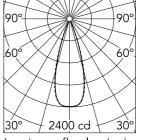
Luminous flux luminaire 768 lm (EXTREME CUT OFF)
