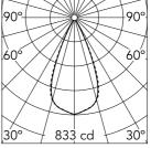
Luminous flux luminaire 452 lm (EXTREME CUT OFF)
