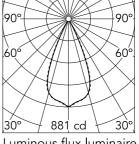
Luminous flux luminaire 464 lm (EXTREME CUT OFF)
