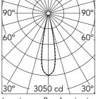
Luminous flux luminaire 453 lm (EXTREME CUT OFF)
