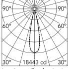
Luminous flux luminaire 2698 lm (EXTREME CUT OFF)
