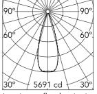
Luminous flux luminaire 1850 lm (EXTREME CUT OFF)
