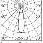
Luminous flux luminaire 788 lm (EXTREME CUT OFF)
