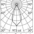
Luminous flux luminaire 467 lm (EXTREME CUT OFF)
