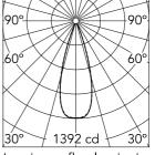
Luminous flux luminaire 447 lm (EXTREME CUT OFF)
