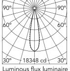
Luminous flux luminaire 2727 lm (EXTREME CUT OFF)
