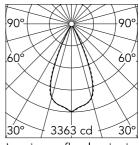
Luminous flux luminaire 1773 lm (EXTREME CUT OFF)
