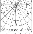
Luminous flux luminaire 1859 lm (EXTREME CUT OFF)
