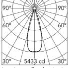
Luminous flux luminaire 1765 lm (EXTREME CUT OFF)
