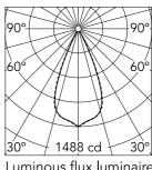
Luminous flux luminaire 784 lm (EXTREME CUT OFF)
