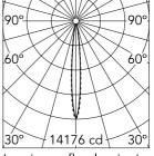
Luminous flux luminaire 805 lm (EXTREME CUT OFF)
