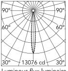
Luminous flux luminaire 724 lm (EXTREME CUT OFF)
