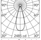
Luminous flux luminaire 803 lm (EXTREME CUT OFF)
