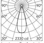
Luminous flux luminaire 752 lm (EXTREME CUT OFF)
