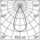
Luminous flux luminaire 452 lm (EXTREME CUT OFF)
