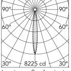
Luminous flux luminaire 465 lm (EXTREME CUT OFF)
