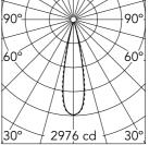
Luminous flux luminaire 445 lm (EXTREME CUT OFF)
