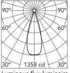
Luminous flux luminaire 441 lm (EXTREME CUT OFF)
