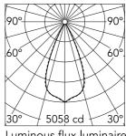
Luminous flux luminaire 2666 lm (EXTREME CUT OFF)
