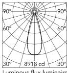
Luminous flux luminaire 2880 lm (EXTREME CUT OFF)
