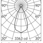
Luminous flux luminaire 1773 lm (EXTREME CUT OFF)
