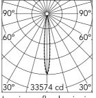
Luminous flux luminaire 1906 lm (EXTREME CUT OFF)
